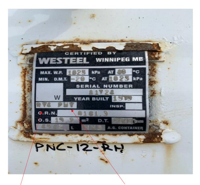
The R/T4 marking is an Engineering Code for welding. The PHT marking indicates Partial Heat Treatment only – The heads are heat treated not the complete tank.
